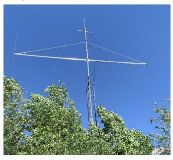
Stations 1,200 miles away have decoded my signal via reflection of my signal off ionized gas produced by small meteorites coming into our atmosphere. They burn up, creating ionized gas, which only lasts a second. WSJT-X encoding on the transmitted carrier is sent hundreds of times per minute and a small amount of data is reflected down to earth which includes my call sign and grid square. It's quite amazing!
