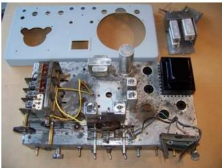
I replaced many capacitors, resistors and all the tubes. You can see the wax coming out of the old capacitors in one of the pictures!
