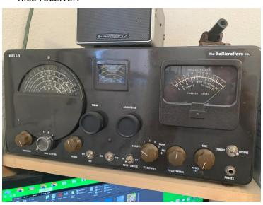
After the restoration I put the old receiver on the air and paired with another old piece of gear, a Heathkit DX-40 transmitter, It ran 50 watts max output and was XTAL controlled.
